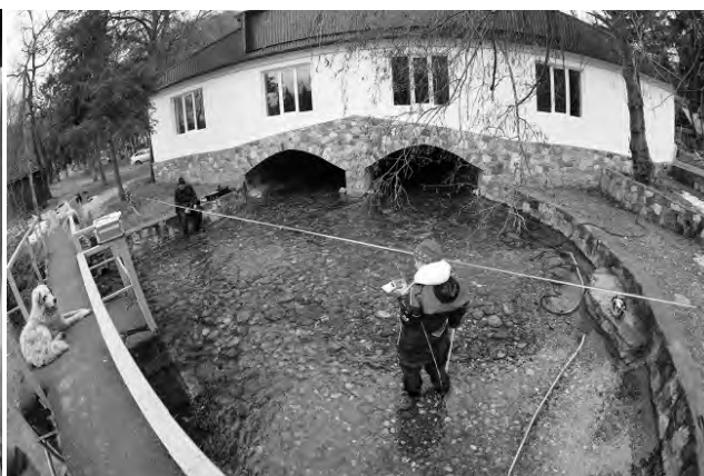
Fig 3. Hydrologic section at the point of Cheric-Kel' lake discharge.
